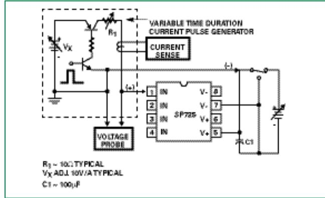
**Figure 5: SP725 Typical Nonrepetitive Peak Current Pulse Capability**
